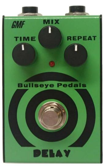
**TIME** knob – This knob controls the delay time. Rotating the knob clockwise will increase the delay time. (140ms – 360ms)
